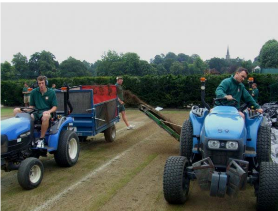
Stripping the grass off the courts with the Koro Topmaker.
